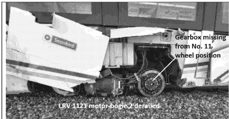
Figure 5. BM2 on LRV 1121 derailed and gearbox missing from wheel position No. 11 (Source: Alstom)
