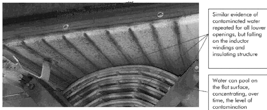
Figure 3.69: Inductor Compartment of a Typical Traction Case, After 75000 km
