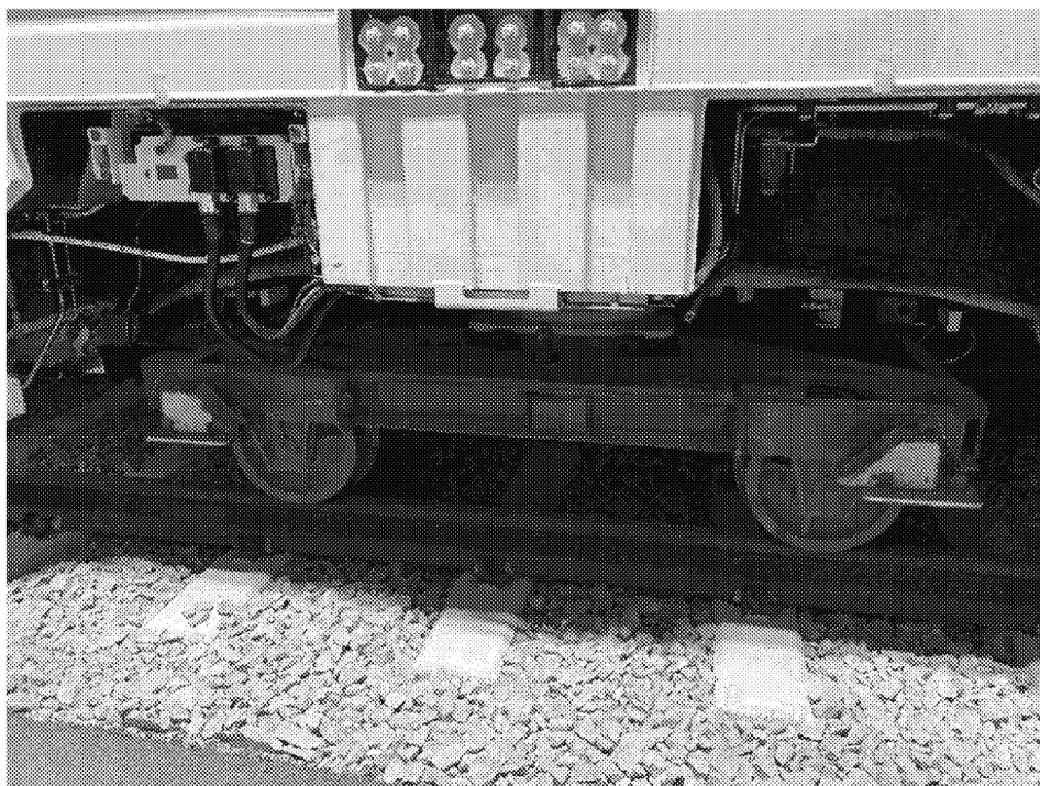
Figure 4.15: Vehicle Missing Trucks
