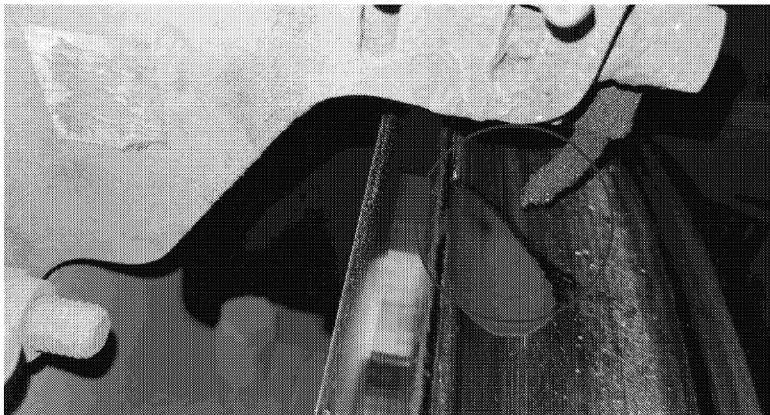
Figure 3.66: Incorrectly Set Flange Lubrication Spray Nozzle
