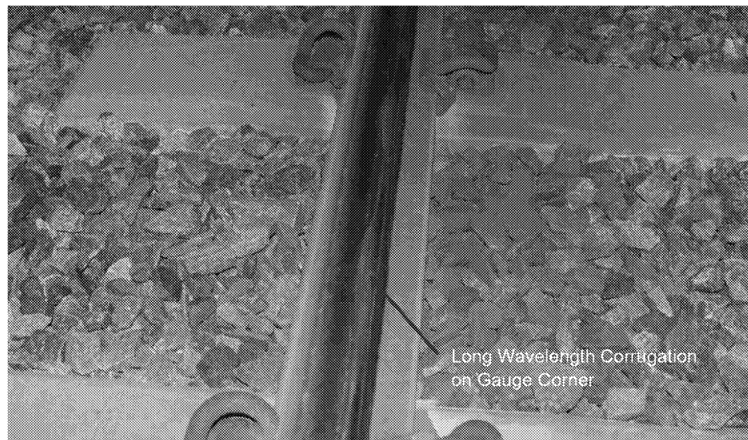
Figure 3.12: Corrugation on High Rail of Curve 330 at 108+685
