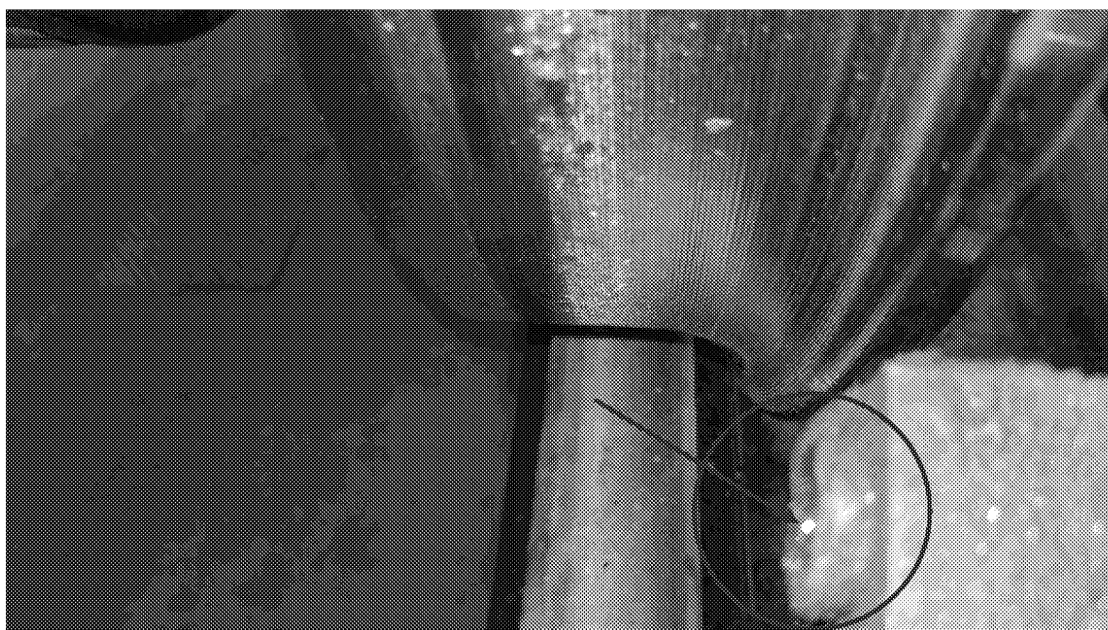
Figure 3.65: Missing Flange Lubrication Spray Nozzle
