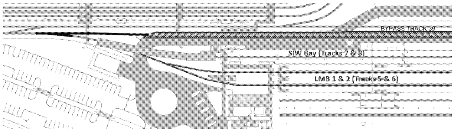
Figure 4.4: MSF1 Access Issue to LMBs 1 and 2 When a Vehicle is Outside the SIW Bay
