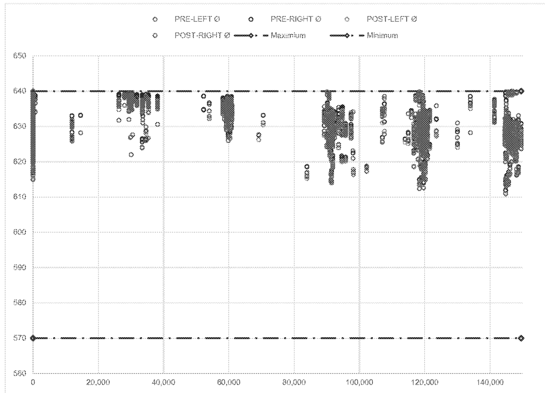
Figure 3.63: Chart of Wheel Diameter Pre and Post Wheel True
