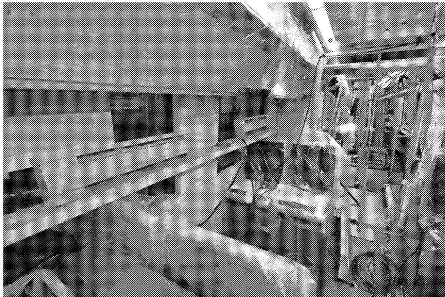
Figure 122 - Resistive Heaters Equally Spaced Throughout LMC2/LCC
