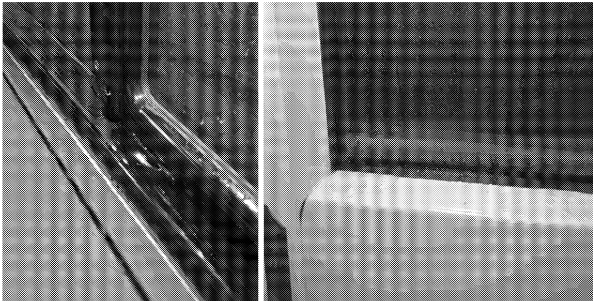
Figure 16 - Water Ingress at Cab Sliding Doors and LMC2 Window
