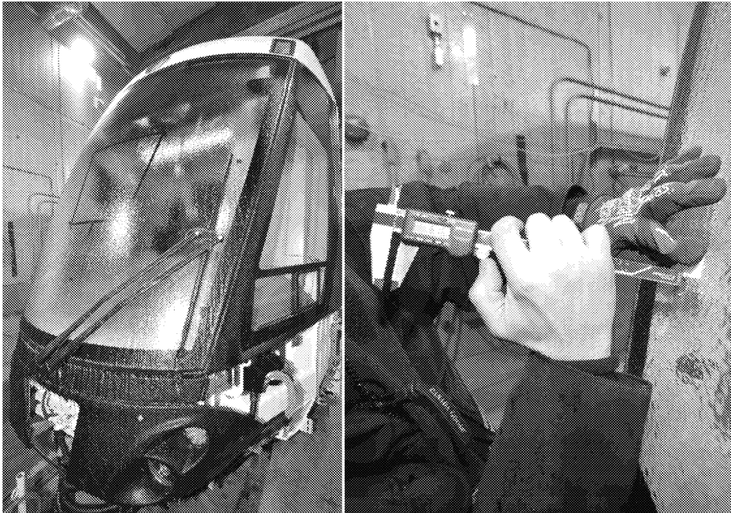
Figure 137 - Ice Accumulation of ~3mm as Measured
