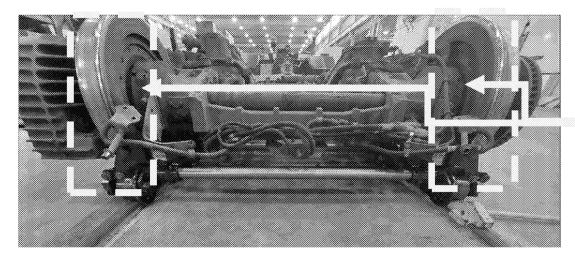
One cartridge bearing assembly (shown below) is the interface between each wheel and the bogie axle
