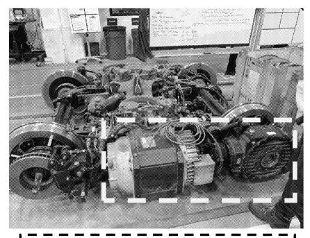
Overhead view of motor bogies (3 per train plus 2 non-motor bogies). Motor and gearbox highlighted.
