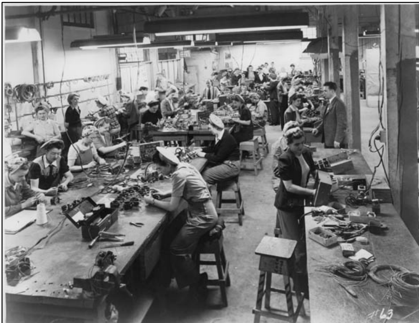
Women soldering and assembling cables for airplanes, Canadian Car and Foundry Co. 1945, Fort William (Ont.). Canadian Car and Foundry Collection. Reference Code: C 190-3-0-0-43 Archives of Ontario, I0002965
